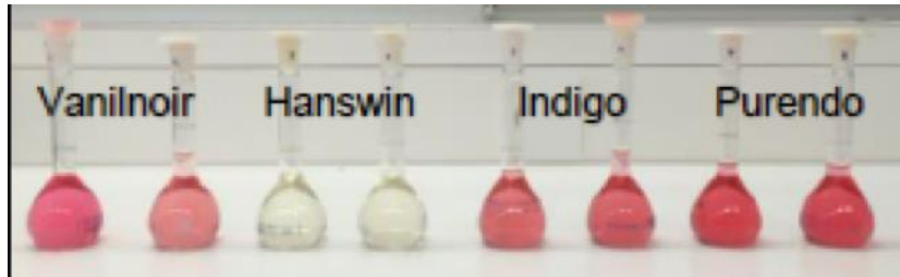
Figure 8. Extraction of anthocyanin compounds in acidified methanol, from whole meal flour of the wheat varieties Vanilnoir, Indigo and Purendo (producing coloured grains), and Hanswin (white grains) (Source: MARTINI Agroscope).
