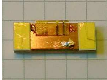
Figure 5.1: Picture of a sample on a submount. The background grid has a spacing of 5 mm. Two stripe contacts were evaporated on the right side of the sample; on the sample's left side, mesa structures were evaporated.
