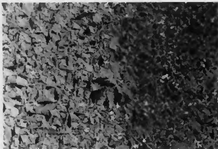
Figure 4.15. Optical Polarised microphotographs of the chiral nematic phase of compound 54 upon cooling from the isotropic liquid at 155°C; 200 x
