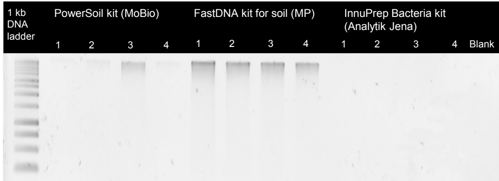
Figure 2.12: Comparison of different DNA extraction kits on an endospore preparations of B. subtilis . The numbers (1, 2, 3 and 4) correspond to the respective extraction cycle. The extraction kits are mentioned on top of the lanes.
