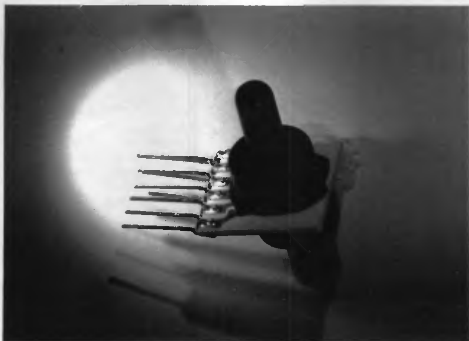
Figure 2.7b: Side view of the completed orifice flow sensor showing the plastic nozzles glued to the ceramic.
