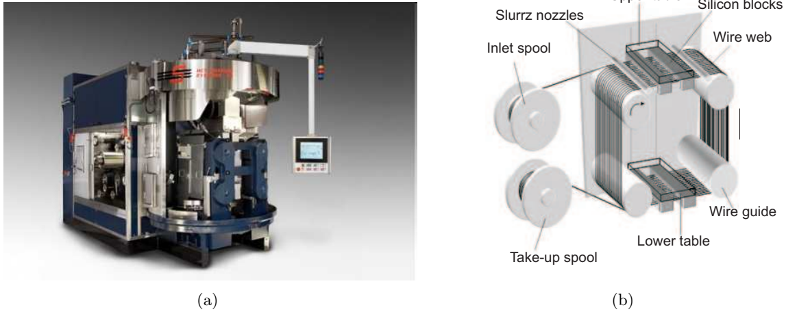
Figure 1.5: (a) A wire-saw from Applied Materials Switzerland SA. (b) Schematic description of a multi-wire slurry saw. The wire-saws usually have two or four wire guides. After Québatte et al 99 . Both images are courtesy of Applied Materials Switzerland — printed with permission.
