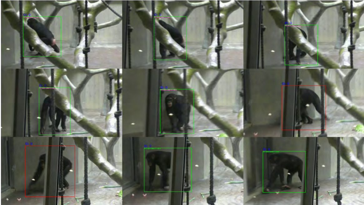
Fig. 4.3 Tracking example after correcting IDs and interpolating missing frames (red bounding box) . When the individual passed behind the pole, the network lost its track and assigned a new ID. All predicted tracks were manually reviewed, and proper IDs reassigned programmatically where necessary. Missing frames were reconstructed using linear interpolation. Best seen zoomed in. Code is available in the project repository.
