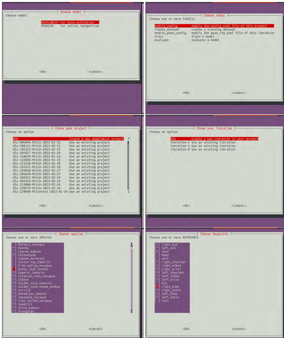
Fig. S4 Examples of UI elements of the ASBAR graphical user interface. The GUI is terminal-based and therefore can be rendered even when accessed on a distant machine, such as a cloud-based platform or a remote high-performance computer.
