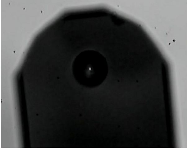
Figure 2.12: Image of the light transmitted through a fully aluminum coated \text{SiO}_2 tip. This top view of the cantilever shows the light emitted from the tip when illuminated with a laser beam from the back.
