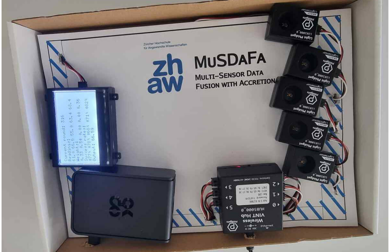
Figure 4.8: Portable 'shoe-box' testbed for our light sensor setup (Figure 4.7). A Raspberry Pi 4 runs the fusion script. An LCD display shows the voting results and weight values.
