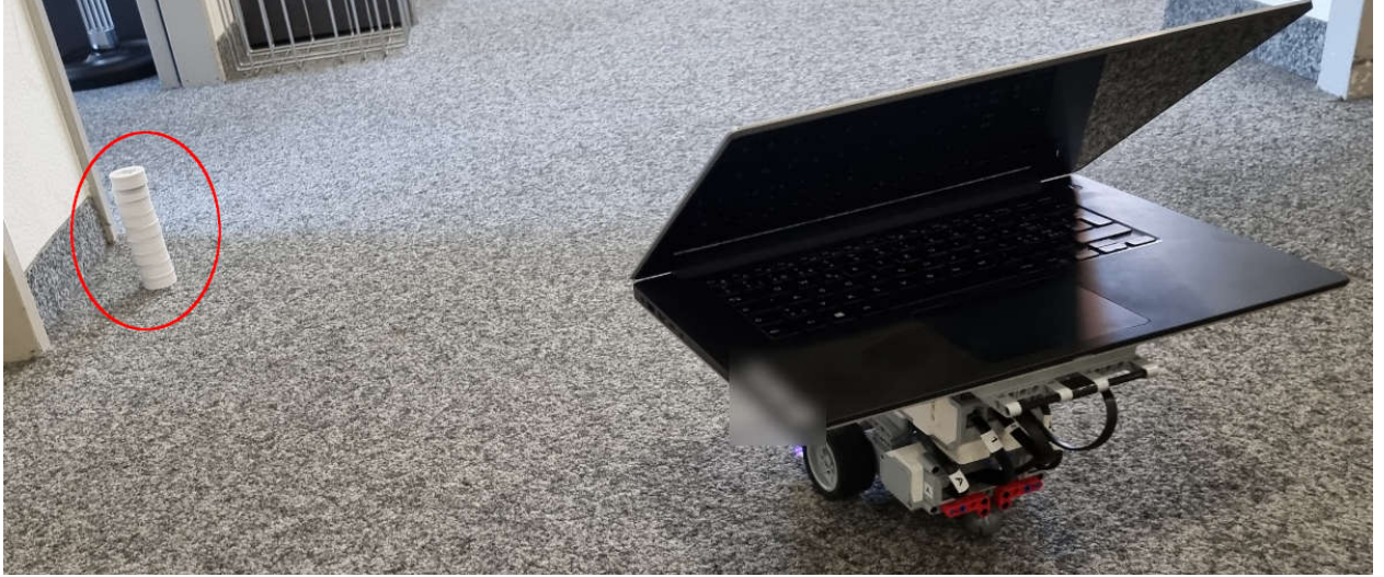
Figure 4.10: Robot driving to the circled beacon stack destination. The laptop acts as bluetooth receiver and edge voter.
