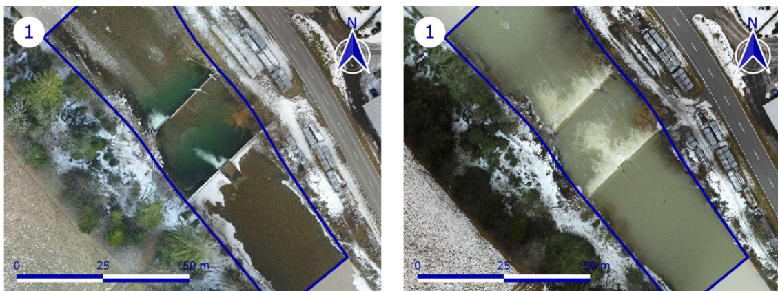
Figure 2.4. View of the simulated couple of weirs of TC1 under different flow regimes.
