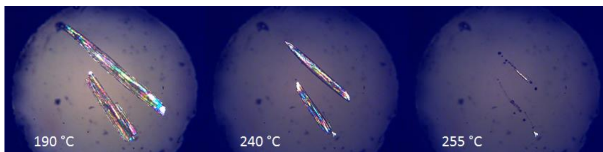
Figure 47. Photos of two crystals of calix-NNNO 11 taken under the microscope at three temperatures: 190 °C (no changes with r.t.), 240 °C (pre-melting was observed) and 255 °C (melting point)
