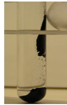
Figure 52: picture of the magnetite formed in FRB enrichment cultures (White object = magnet).
