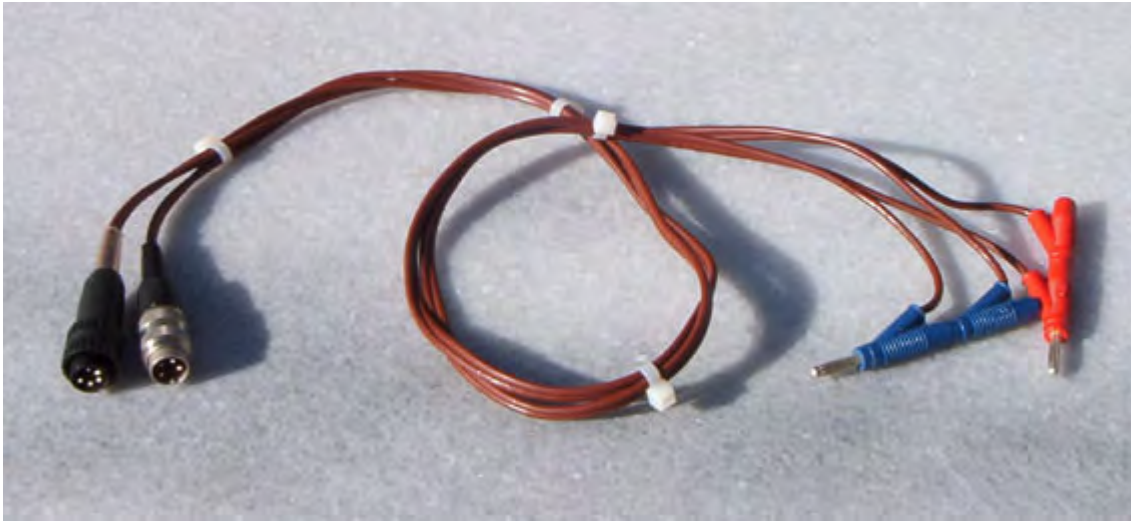
Fig. A - 10: Cable 4: for charging the Battery-Pack. Use chargers for PB Accus!
