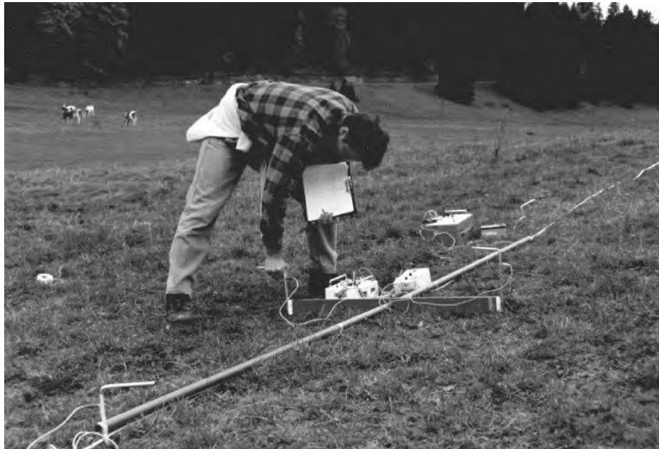
FIG. 3. Geoelectric null-array measurement (Schlumberger null-array) in the field. A plastic tube with a proper length and a wooden lattice fixed on it serves to reduce geometrical errors.
