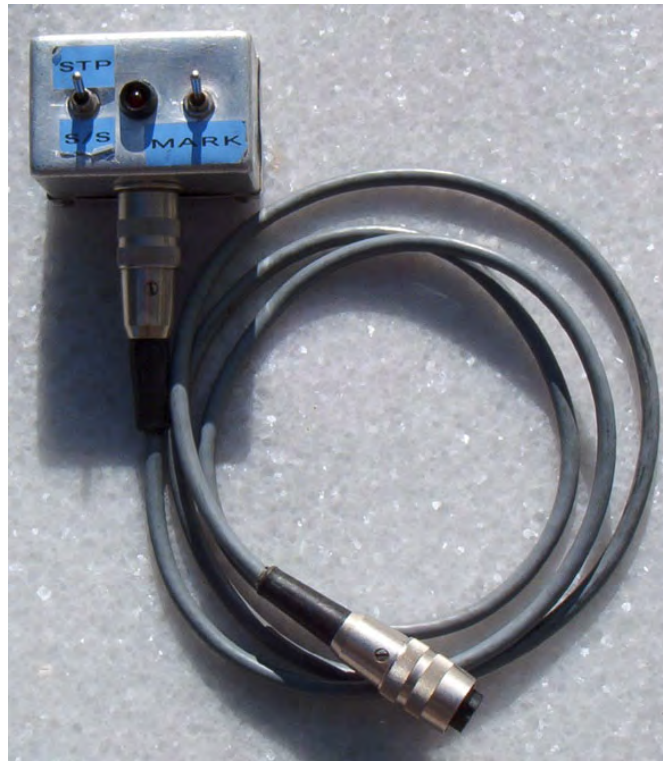
Fig. A - 4: Datalogger RemoteControl with cable. Box (from left to right): (1) Switcher position "STP" = STOP, "S/S" = RECORD; (2) LED; (3) Switcher "MARK"
