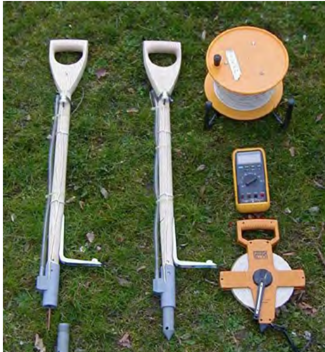
Figure 12 Self-potential field equipment "Type Münster" consisting out of two \text{Cu-CuSO}_4 electrodes mounted on spade sticks, volt-meter, tape-measure, cable.
