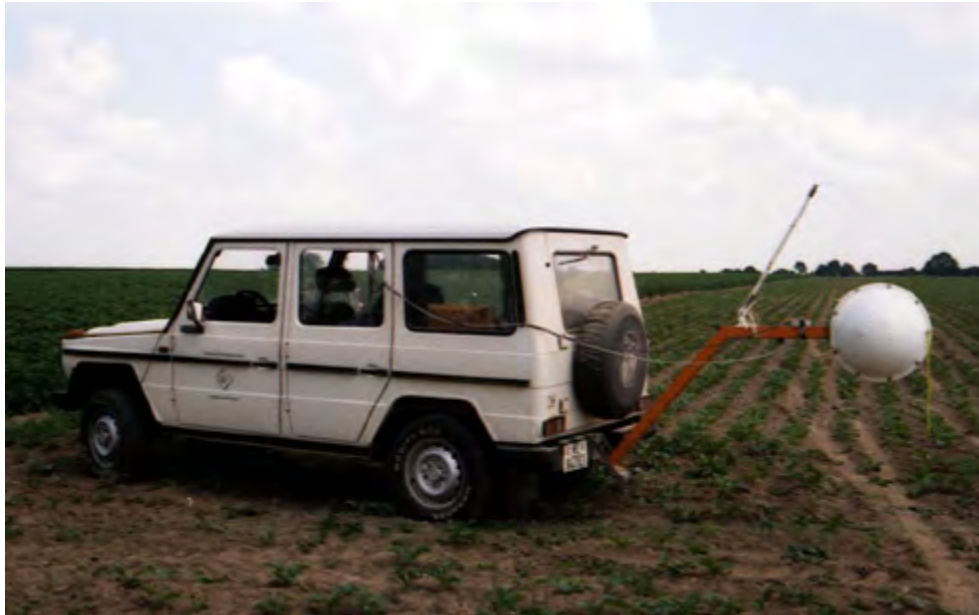
Figure 10 RF-EM system with selforientating antenna fixed behind a car.
