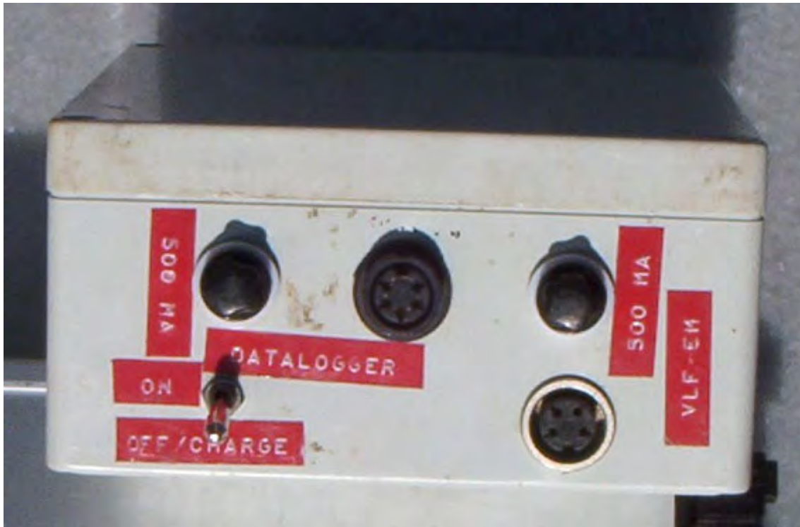
Fig. A - 6: Front panel of BATTERY-PACK with "ON/OFF Switcher", Fuses and Sockets for power supply cables to DATALOGGER and RECEIVER. Pack includes two 12 Volt PB Accus.
