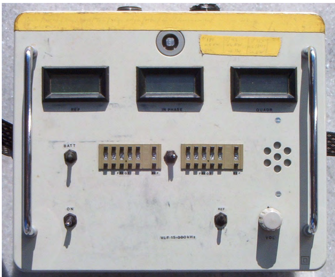
Fig. A - 2: Front view of RF-EM receiver. Two different frequencies can be pre-tuned. Switcher "REF/MOT" has to be in position "REF" while measuring.
