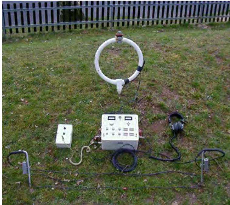
Figure 8 The RMT equipment (12-240 kHz). Components from top to bottom and left to right: magnetic induction coil, battery, receiver-unit, headphones, electrodes.
