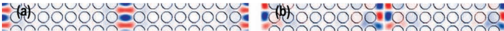
Figure 9: Plane wave expansion simulation showing mode patterns within the PhC waveguide. The modes were calculated using an approximate supercell-based model of the ideal structure. The two lowest-order eigenmodes are shown: (a) even mode e_1 ; (b) odd mode e_2 .
