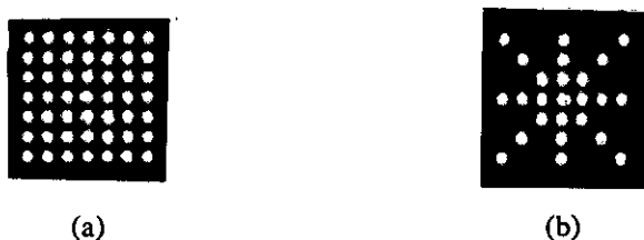
Fig. 2.4 The N \times N diffraction orders of equal intensity (a) and the resulting input neural matrix after modulation (b).
