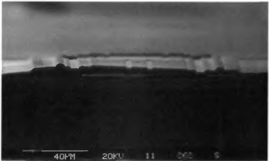
Figure 2.5: SEM of a polysilicon beam encapsulated by a second polysilicon cover; the distance between cover, beam and substrate are 2.2 \mu\text{m} and 1.8 \mu\text{m} respectively.
