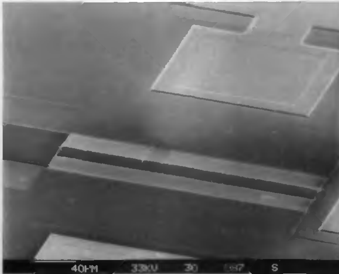
Figure 4.2: SEM of a 350 \mu\text{m} long microrelay.
