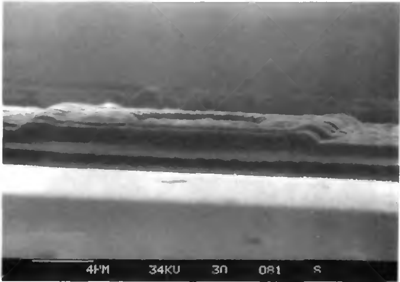
Figure 3.7: SEM of the micro-bump providing an improved electrical contact between both conductors of the working circuit.
