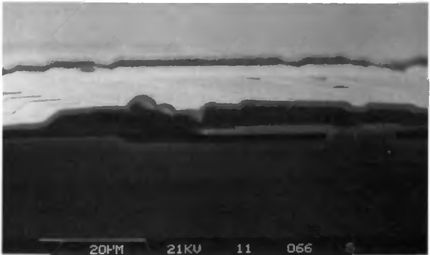
Figure 2.6: SEM close-up of a polysilicon beam encapsulated by a second polysilicon cover; the distance between cover, beam and substrate are 2.2 \mu\text{m} and 1.8 \mu\text{m} respectively. Note that the beam was not completely released.
