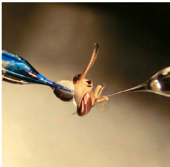
Figure 2.1: Picture of a G. pallidipes head prepared for EAG recordings. The head is removed from the body and mounted between the reference electrode painted in blue and the measuring electrode placed at the tip of the funiculus. The reference electrode crosses the occipital condyle and arrives at the base of the antenna.
