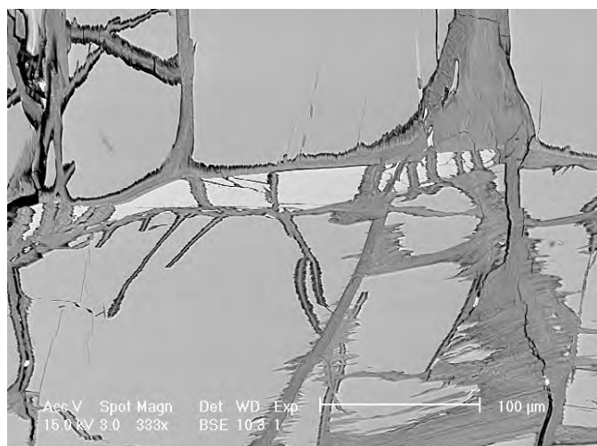
Elongated cpx grain between opx (with exsolution lamellae) in serpentine
