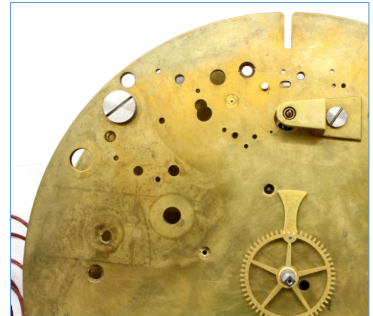
Detail of the traces of an old unknown device present on the plate of the Winnerl sidereal clock
