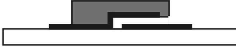
Figure 3.25: Electrostatic cantilever beam parallel plate actuator. For the calculations, it is assumed that the electrodes are covering the whole length and width of the cantilever beam.
