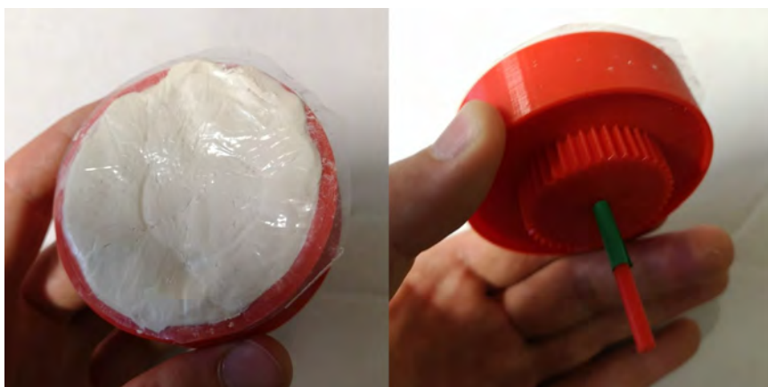
Figure 5.8: 3D printed part for rotating a mineral sample.
