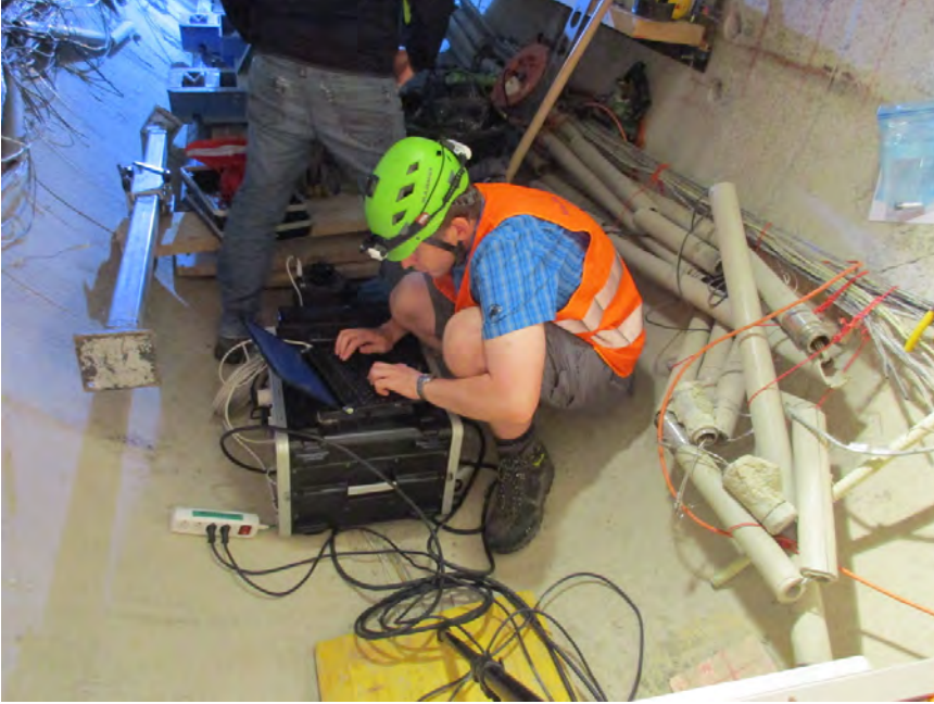
Figure 5.3: Example of working conditions in the Grimsel underground laboratory. The control laptop (which has the GUI) is laid on top of the box containing the camera power supply, the server and the frame grabber.
