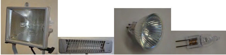
Figure 2.5: Light sources investigated. From left to right: 230V AC 300W halogen flood light, 230V AC quartz heater, 12V DC 30W halogen lamp with reflector, 12V DC 30W halogen bulb.
