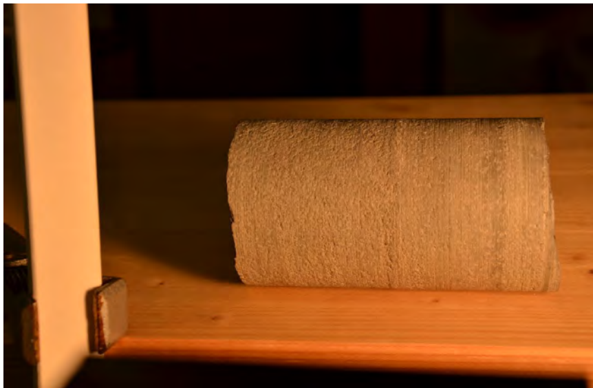
Figure 2.11: Sample as seen from the camera. The core has a diameter of 7cm, and is 12cm long. The support is made of Epicea wood.
