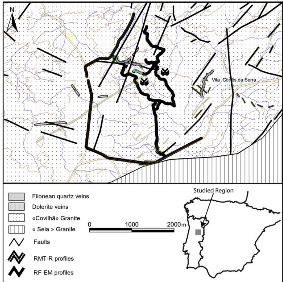
Fig. 21 Geological settings and location of the geophysical survey (RF-EM and RMT) carried out in Castelejo. Table 4 (ESM) indicates natural and artificial constraints for the EM surveys
