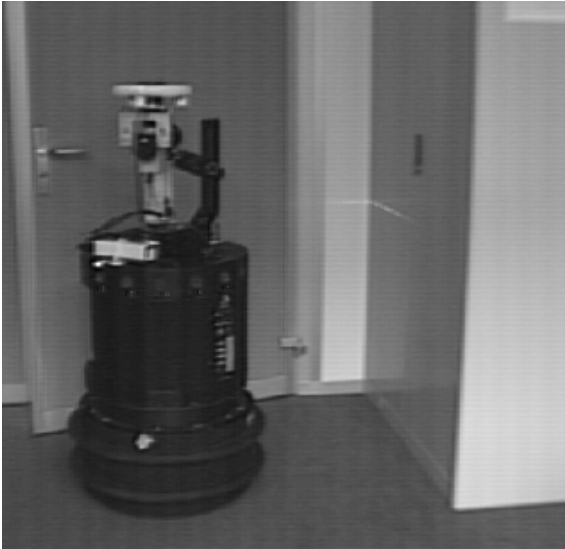
Figure 2: Self-positioning the robot by homing on a corner
