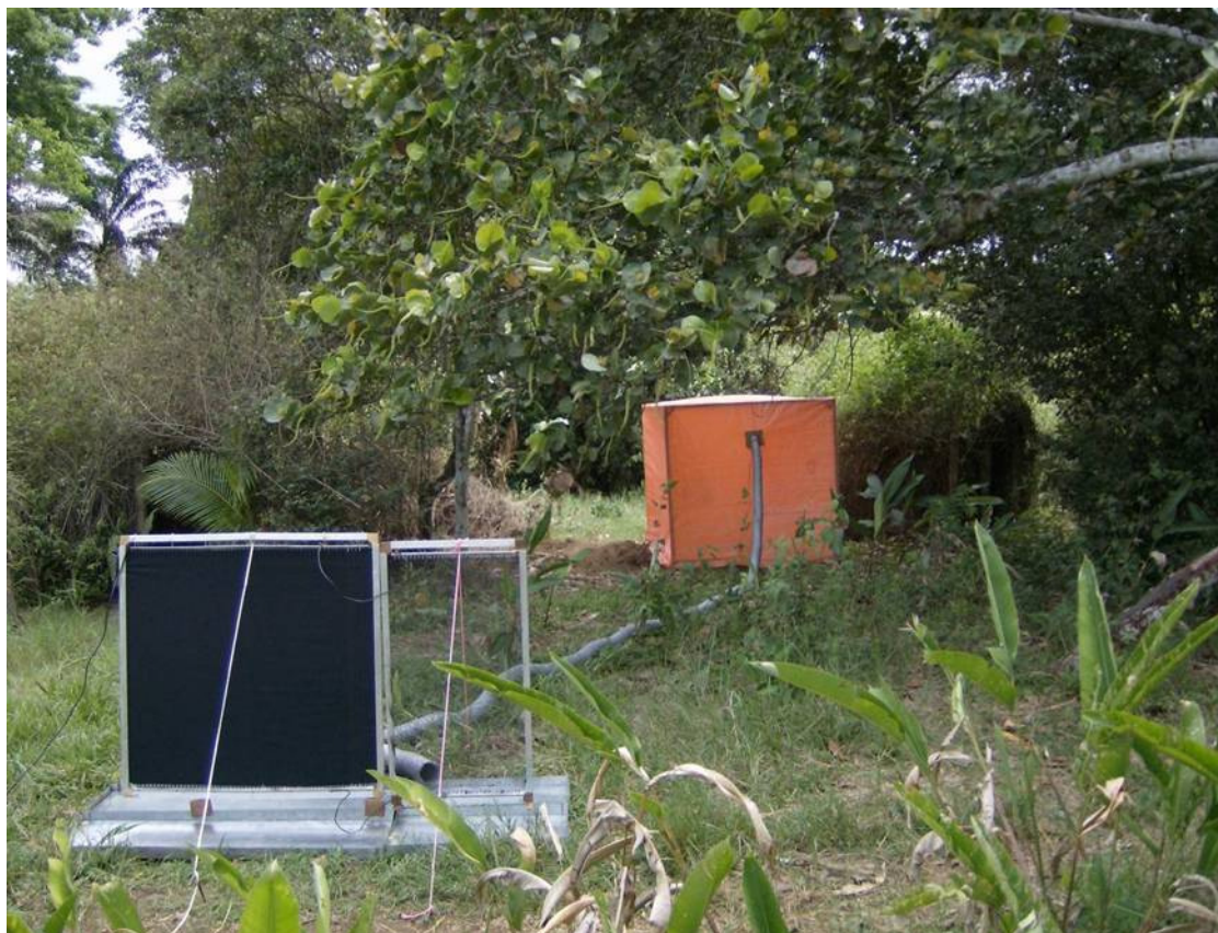
Figure 1B. E-target with flanking E-nets. The grey pipe leading up to the trap or target carries odour-laden air from a tent, visible in the background, containing live hosts.
