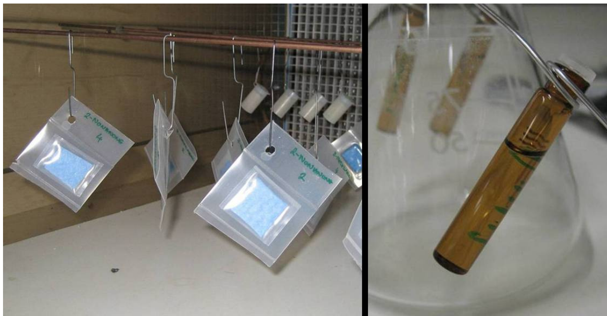
Plate 1: Sachets, polyvials and Chromacol used as dispensers of chemicals during the field trial
