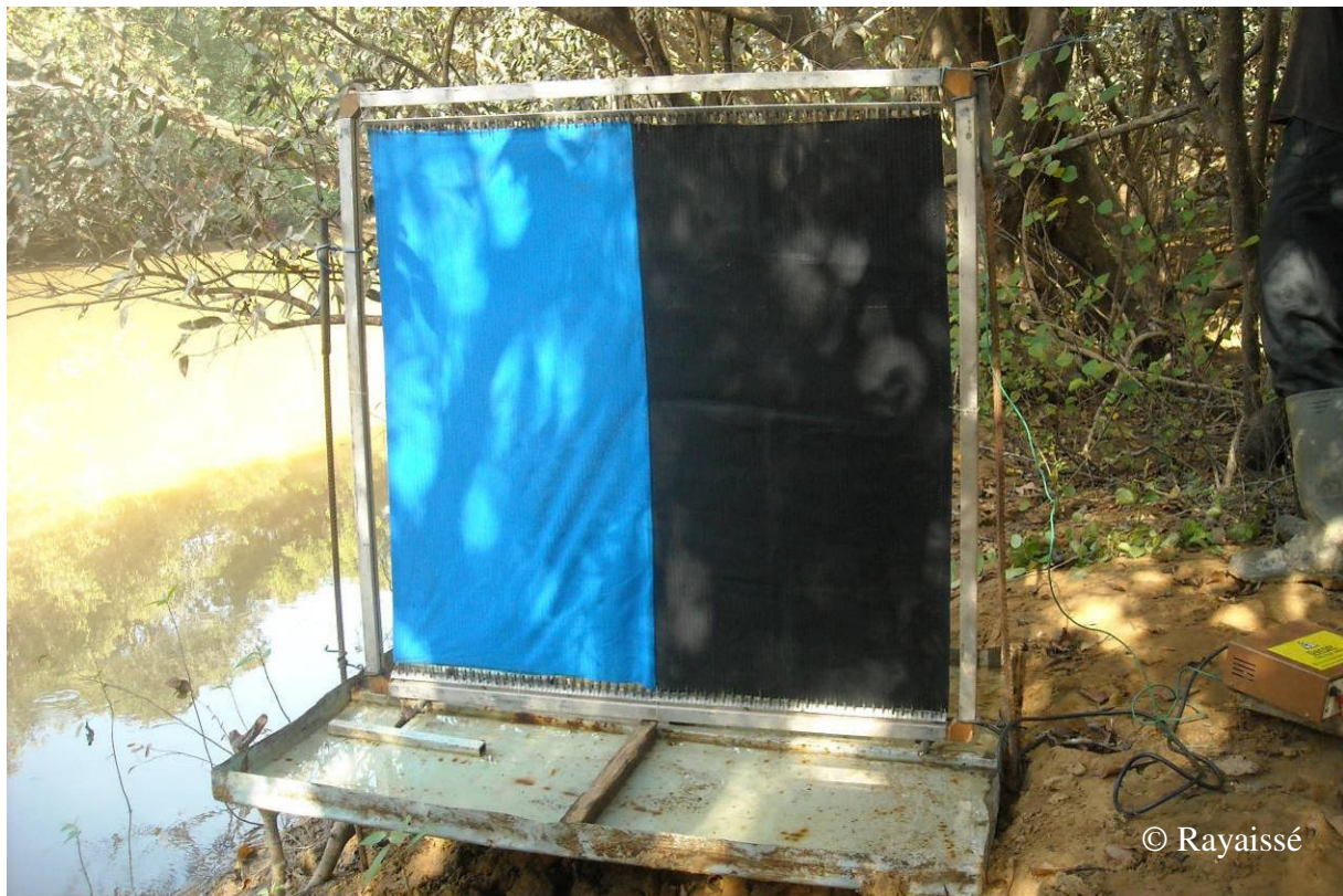
Plate 5: A blue/black target set on a tray with separate portions for collection of flies according to the colour of the cloth
