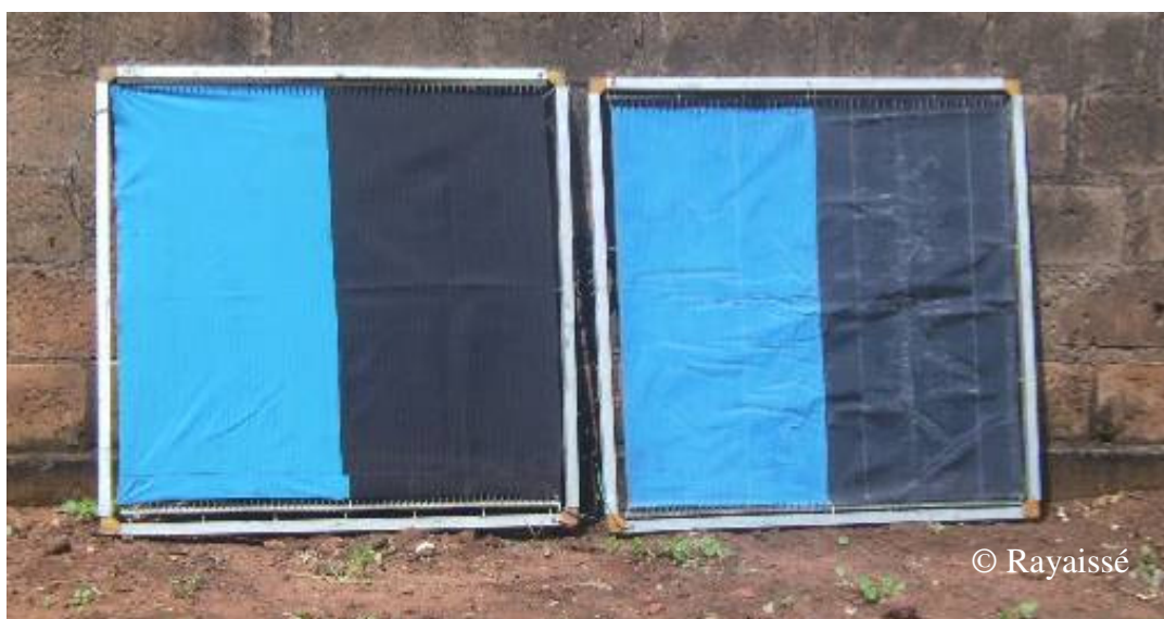
Plate 4: A matt target (treatment A) and target covered with shinyfilm with the shiny side facing outwards (treatment B) inserted between electric grids
