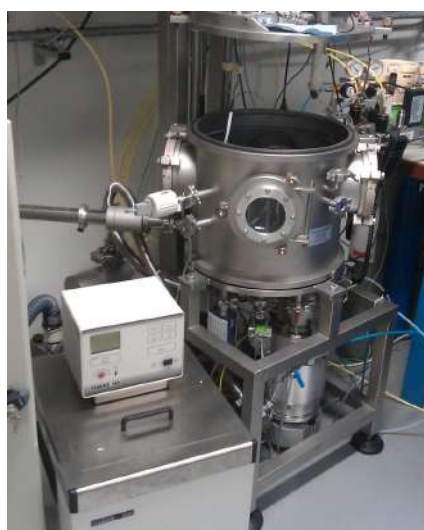
(B) LTF-SAMLAB micro-fabricated cell filling system (co-owned equipment by UniNE and EPFL). Courtesy: Y. Pétremand.
