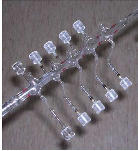
FIGURE 5.1: Parylene ramp before being filled with rubidium.
