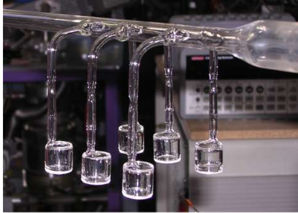
FIGURE 3.2: Typical cell ramp mounted on our cell filling system.
