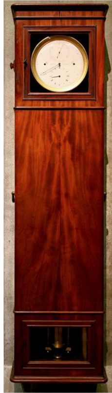
Figure 6. Winnerl sidereal pendulum clock in its case, preserved at the MIH.
