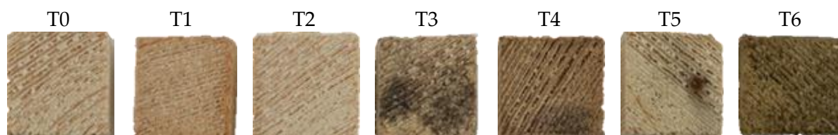
Figure S 1: Pine wood samples, either untreated (T0) or after degradation protocol (T1: H 2 O+vacuum; T2: UV; T3: N 2 +vacuum; T4: H 2 O 2 :NH 4 OH; T5: T1+metal; T6: fungi)
