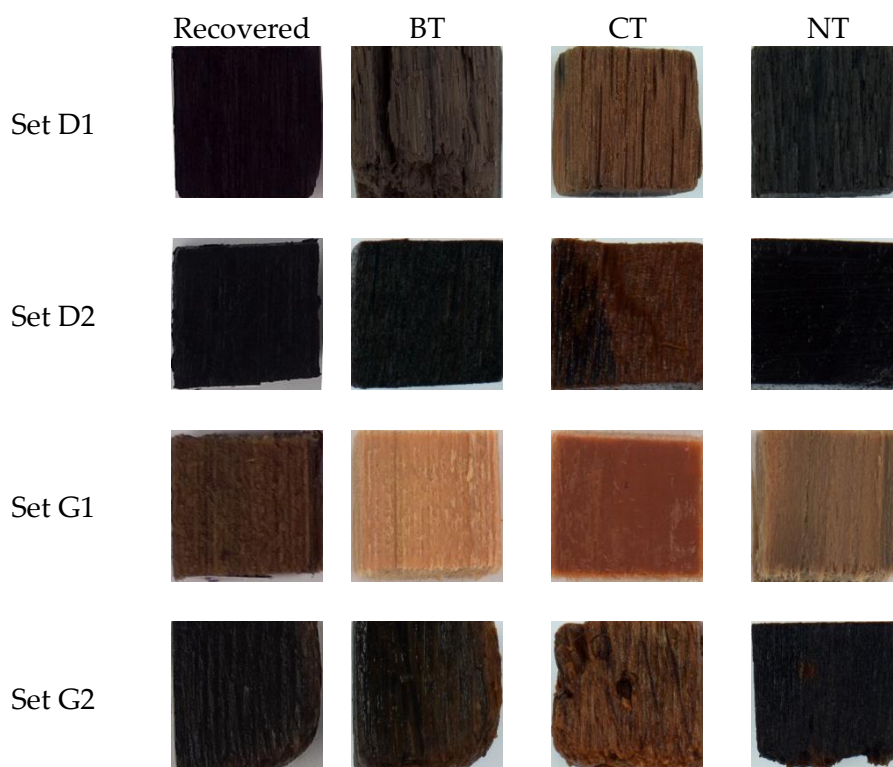
Figure 31: Visual appearance of model archaeological oak (sets D1, D2 and G2) and pine (set G1) as recovered and after extraction with biological (BT) and chemical (CT) method compared with untreated (NT) samples
