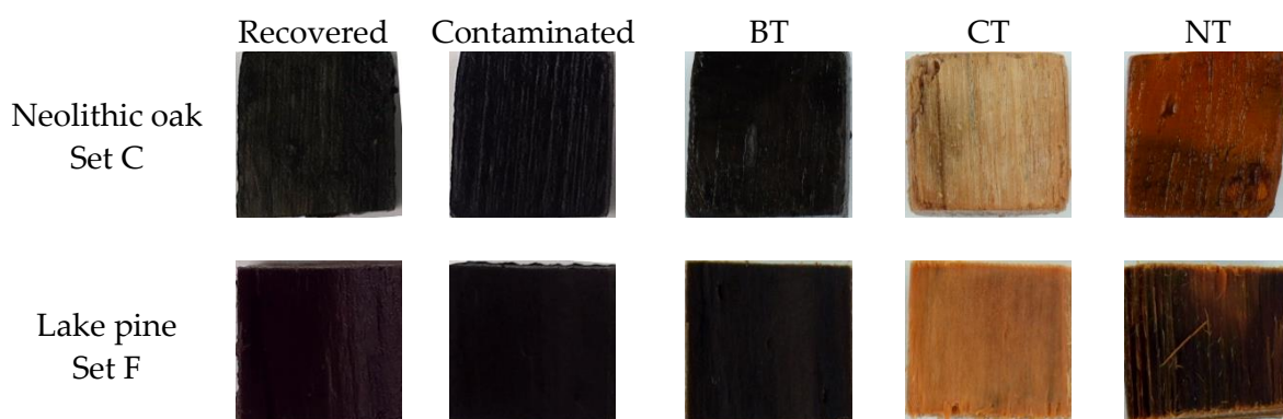
Figure 30: Visual appearance of model oak (set C) and pine (set F) as recovered, after contamination with IP1 and after extraction with biological (BT) or chemical (CT) method compared with untreated (NT) samples
