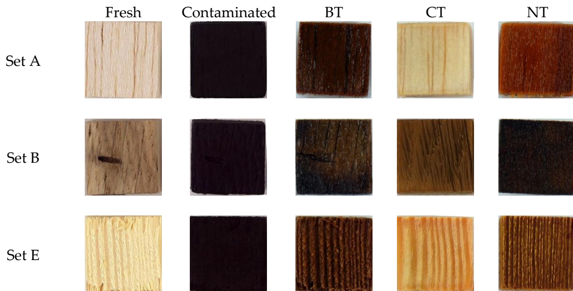
Figure S 11: Visual appearance of fresh balsa (set A), oak (set B) and pine (set E) as fresh, after contaminated with IP1 to simulate WAW and after extraction with biological (BT) and chemical (CT) treatments compared with untreated (NT) samples
