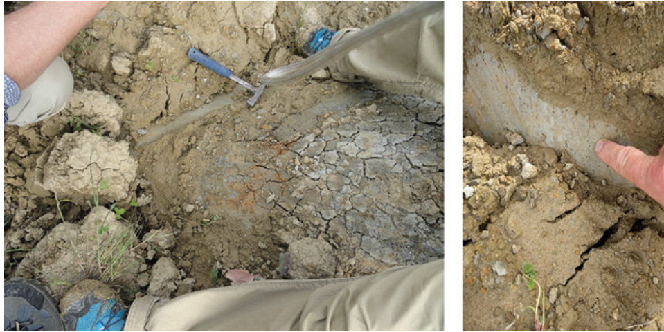
Figure 9.4 Left: looking vertically down at a landslide scarp in the Collazone study area, Italy, showing how the slid material in the top of the image has smoothed underlying, uneroded material into a thin clayey layer. Land-sliding here happened in different phases over a few days, and as a result the earliest exposed smooth layer to the right has already cracked when drying out in the air. The most recently exposed smooth layer left of the hammer is still smooth, as unexposed layers probably are as well. Right: Zoomed in to the recently exposed smooth layer, showing smooth, parallel clay minerals. (Courtesy of Arnaud Temme.)
