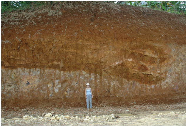
Figure 7.1 Soil profile developed in a weathering volcanic debris deposit in Guadeloupe. Note the presence of weathering clasts that are distinguished by color.
