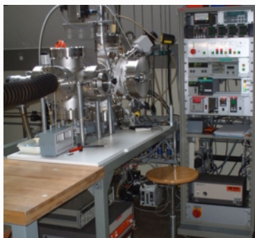
Fig. 1.1: Image of the PE-CVD deposition vacuum chamber 'System G' used for the fabrication of \mu\text{c-Si:H} n-i-p solar cells.
