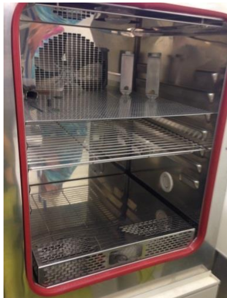
Figure 17. Climatic chamber used for the ageing procedures on LAT samples showing the aluminium trail covered with a micro-perforated plastic film
