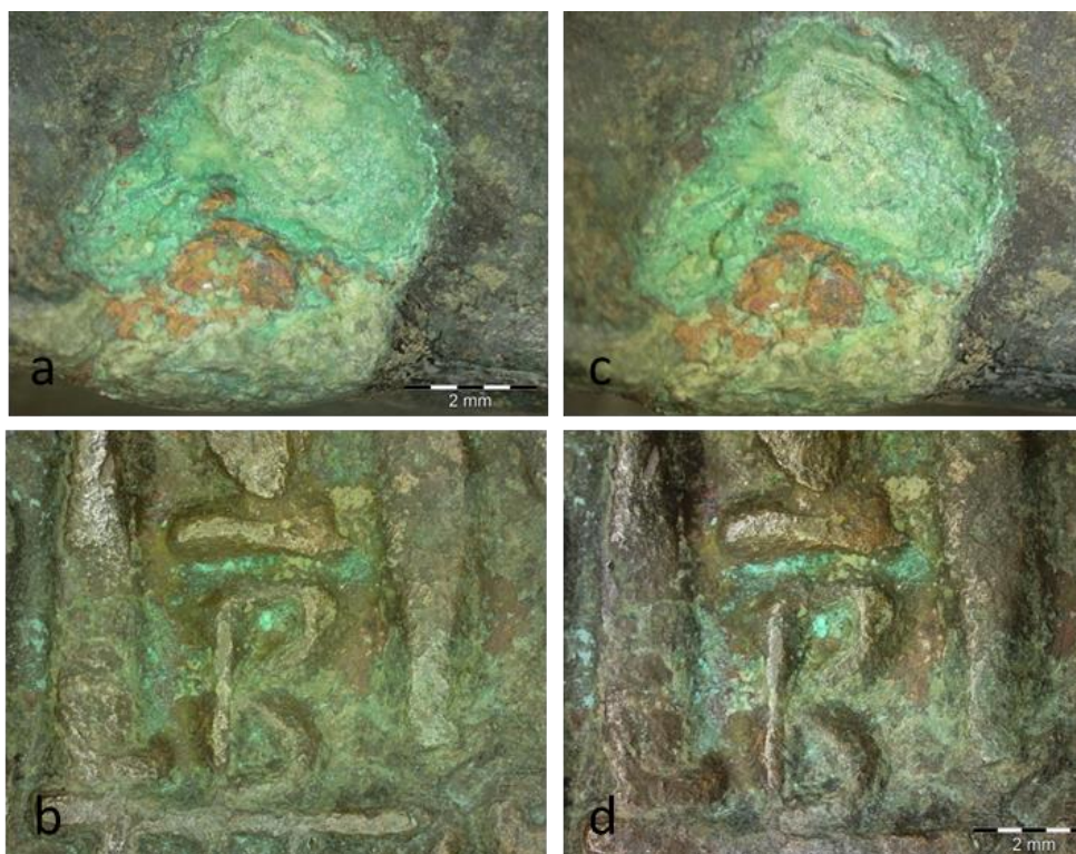
Figure 31. Biopatina-treated objects F23 and A5 before ageing (a-b) and after ageing (c-d) respectively. No significant visual changes
