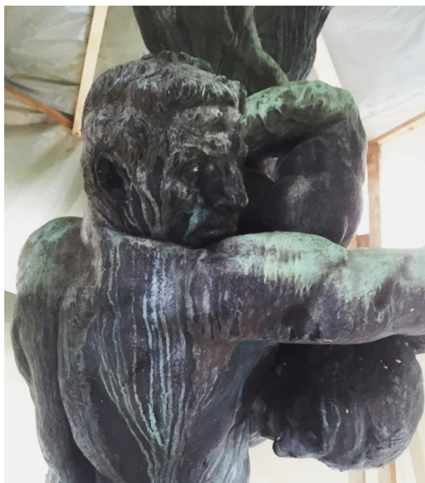
Figure 76. Statue “Schwinger” (Siegwart 1905) located in Lucerne before restoration intervention (2015) showing vertical light green streaks characteristic of unsheltered areas
