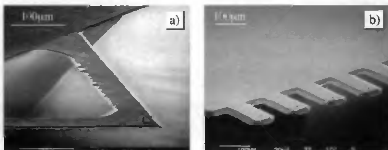
FIG. 3.3: SEMs of completed AFM probes. a) A 2.9\mu\text{m} thick V-shaped cantilever made from a SOI wafer and b) an array of 9\mu\text{m} thick beam cantilevers made from a standard wafer, for applications needing a high spring constant.
