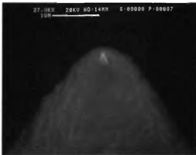
FIG. 5.5: SEM of a partially released diamond tip pointing out of the silicon nitride layer remaining after a combination of dry etching ( \text{SF}_6/\text{O}_2 , 8min) and wet etching ( \text{H}_3\text{PO}_4 , 180°C, 45 min). The base diameter of the boron-doped diamond tip apex not passivated by the insulating layer is 220nm, its height about 300nm, while its radius of curvature is estimated to be smaller than 20nm. Such structures could be used as ultra-precise nanoelectrodes or nanoprobes.
