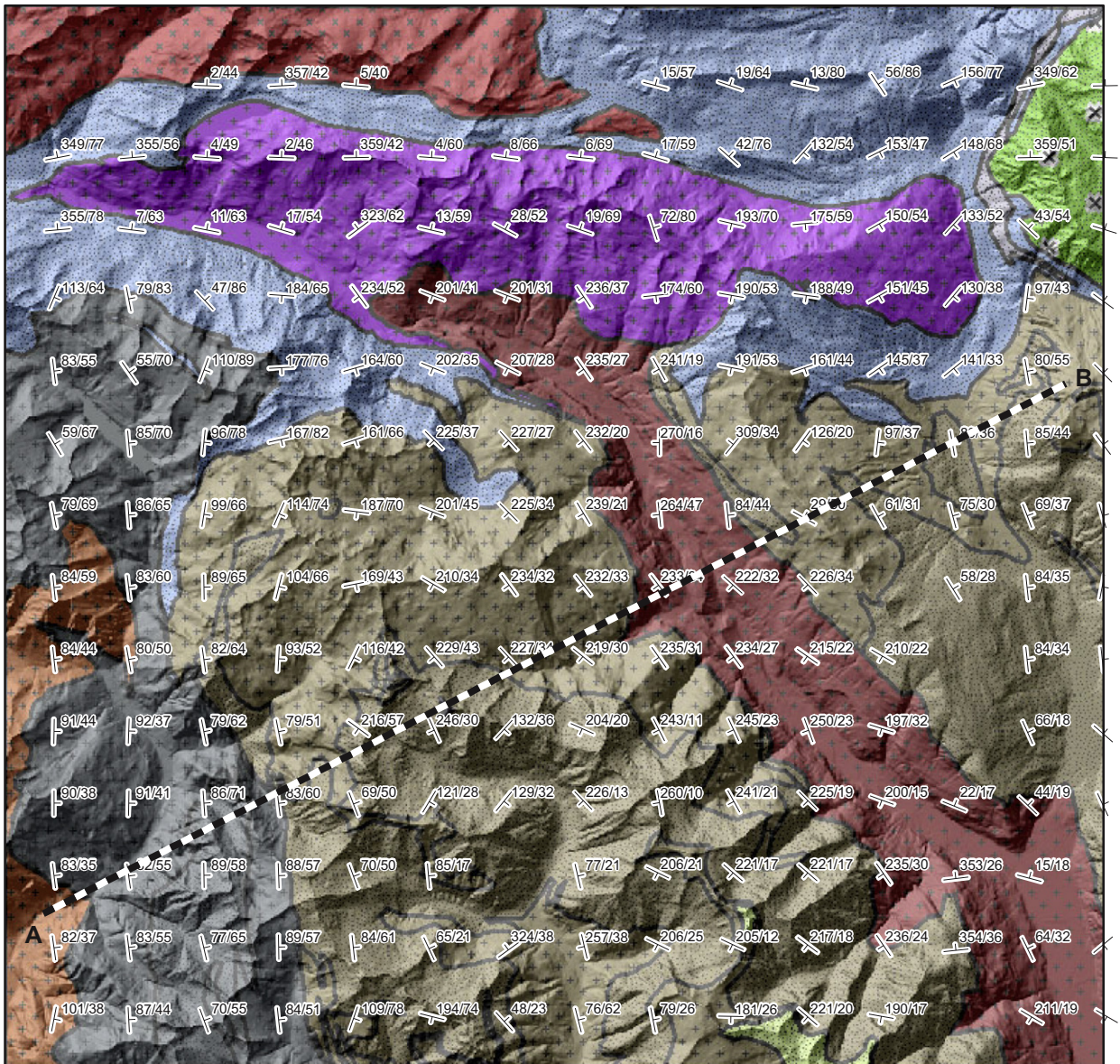
Fig. 5. Inset of a tectonic map from the Central Alps of Switzerland (simplified after Preiswerk et al., 1934), combined with a hill shade calculated from corresponding DEM. Easier correlation of outcrop lines in space (compared to standard map views) facilitates a first visual three-dimensional assessment. Orientation data are spatially averaged from a set of 2964 measurements with the VBA macro Profile Calculation (see footnote 1). SW–NE trending line indicates location of cross-section shown in Fig. 7.
