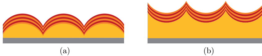
Figure 1.3: Illustration of a multilayer reflector coated on: (a) a microlens array, (b) a concave microlens array.
