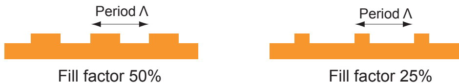
Figure 7.14: Definition of the fill-factor for the grating structure.
