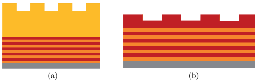
Figure 1.4: Illustrations of a combination of a multilayer Bragg reflector and a corrugated grating with: (a) a thick layer between grating and multilayer; (b) a thin layer between grating and multilayer.
