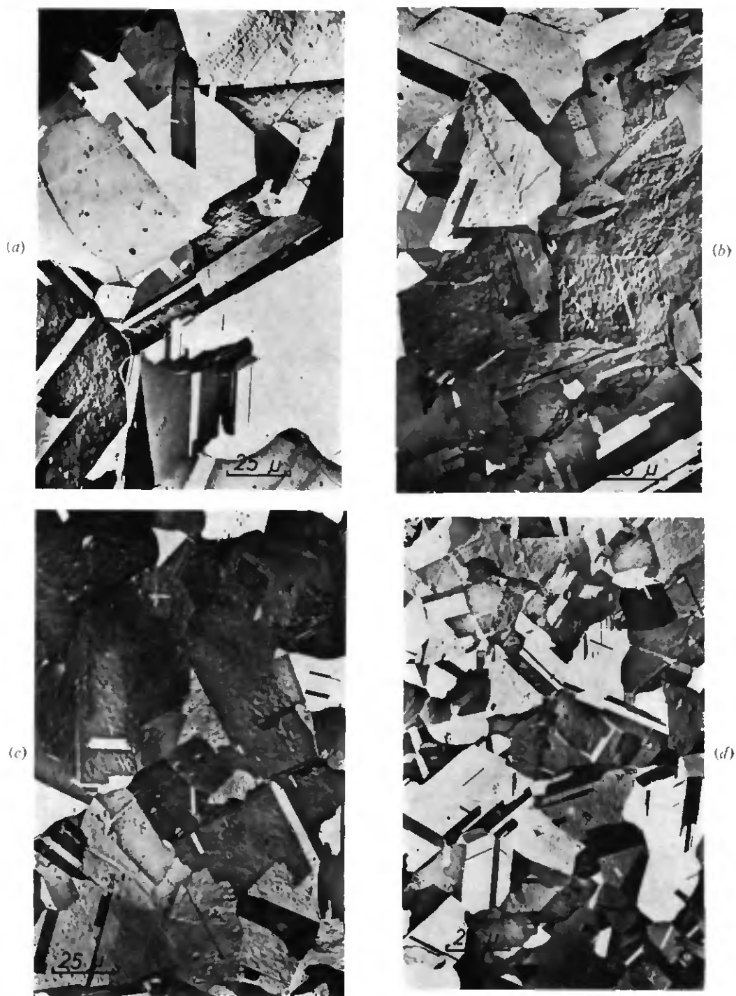
Fig. 10 Electron micrographs of the four copper samples in the fully recrystallized state. The pictures are arranged in the order of decreasing grain size: (a) CA 41; (b) CA 44; (c) CA 42; (d) CA 43.
