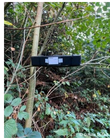
Figure 2: Footprint tunnel with informative label.
