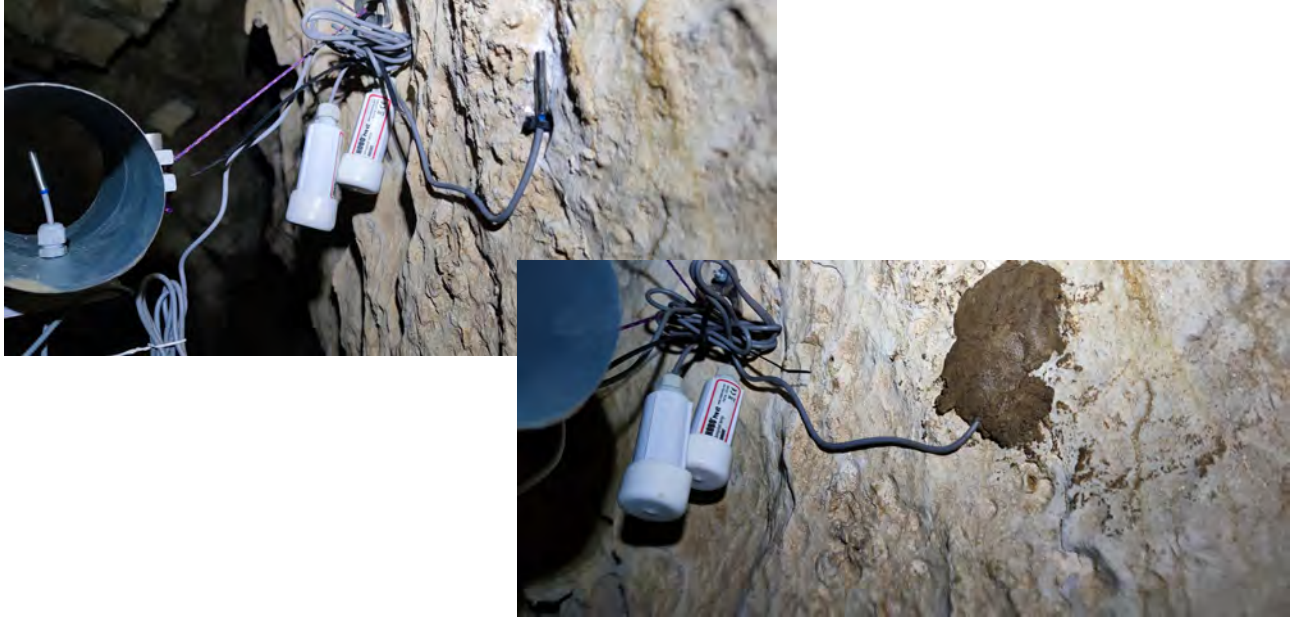
Figure 3.2 – Monitoring setting for the radiative experiment at station T7 in Longeague Cave, with TMCx probes measuring both air and wall surface temperatures.
