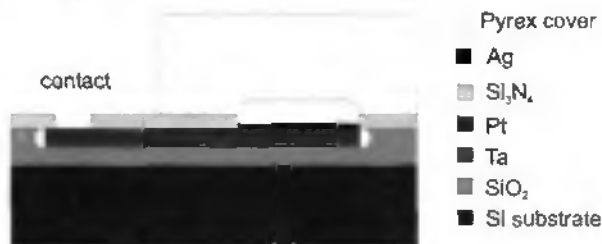
Fig.2.8. Cross-section of the coulometric nanotitrator equipped with a glass channel
