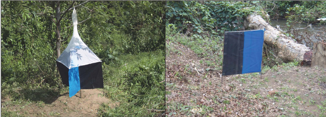
Figure 2. Pyramidal trap and regular 1 m 2 blue-black target with adhesive film in gallery forest, Tabi, Angola. doi:10.1371/journal.pntd.0002601.g002
