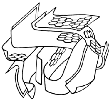
Figure 1. Possible model for the structure of activated carbons, where the micropores correspond to slits between locally parallel aromatic sheets (reprinted from [1,12]).
