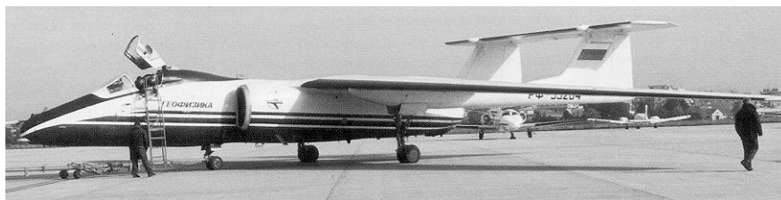
Figure 6.1. The Russian M-55 “Geophysica” high-altitude aircraft. The dorsal bays were removed at the time of this view.
