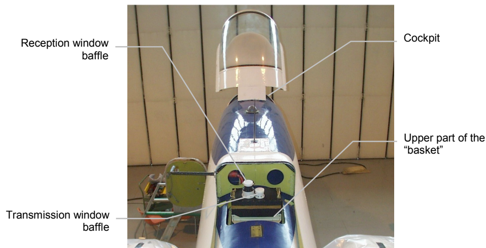
Figure 6.9. GMAL instrument installed on board the “Geophysica” aircraft
