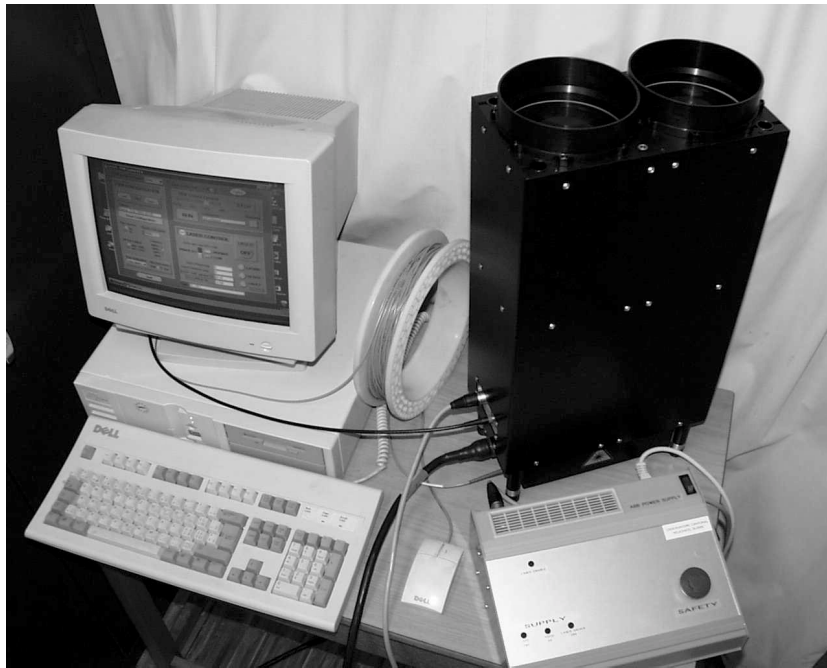
Figure 4.1. View of the compact PRN-cw total backscatter lidar (ABB). Counter-clockwise from right up: the optical package, the optical fibre link, the computer with the PRN generator and the acquisition boards, the DC power supply unit. The desktop computer has been replaced by an industrial computer connected to a laptop in the final configuration.
