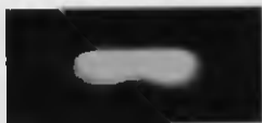
Fig. V.21 Photograph of the waveguide output, with the input spot located at the waveguide centre, with a symmetric output intensity distribution, denoting the correct adjustment of the input beam incidence angle Multimode waveguide width: 18 \mu\text{m}
