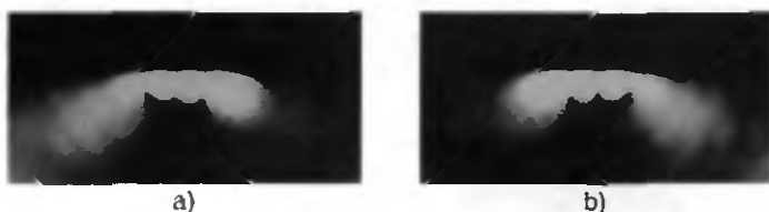
Fig. V.20 Photograph of the waveguide output, with the input spot located near the right side of the waveguide (a), and near the left side (b).
