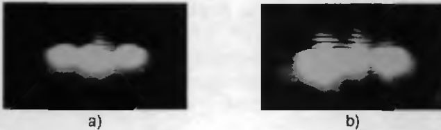
Fig. V.25 Picture of the output intensity distribution, a) with the input spot located in the central branch and, b) located in a side branch of the three-branch coupler
