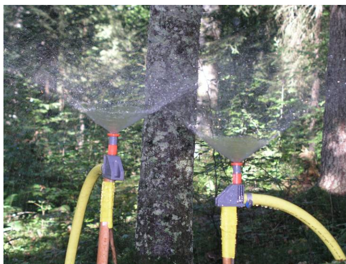
Figure 2.12. Rainmaking device constructed with sprinkler traditionally used for garden watering.
