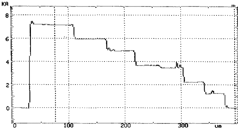
Fig. 7.3.1-2 Etch profile of DOE after final etching step
