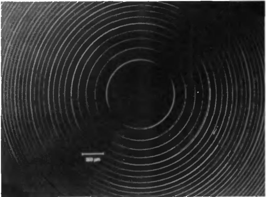
Fig. 6.2.2-11 Microphotograph of DOE structure (differential interference contrast, incident light)
