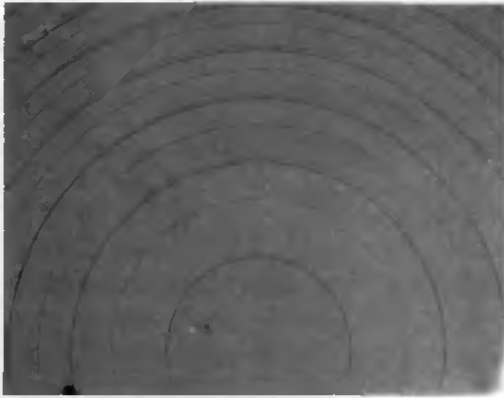
Fig. 6.2.2-8 Mask misalignment effect on DOE structure
