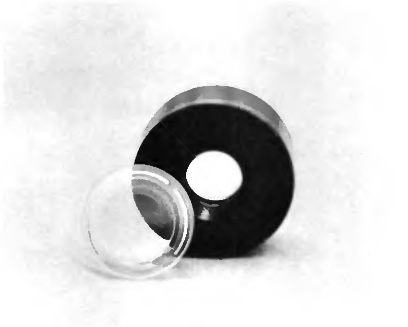
Fig. 6.2.3-6 Hybrid lens and reference lens mount
