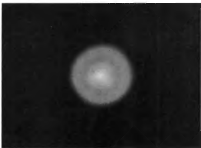
Fig. 7.3.2-7 Airy spot photographs in white light and defocused conditions: (a) cemented achromat 1:2.3, (b) hybrid HY6 1:1.8
