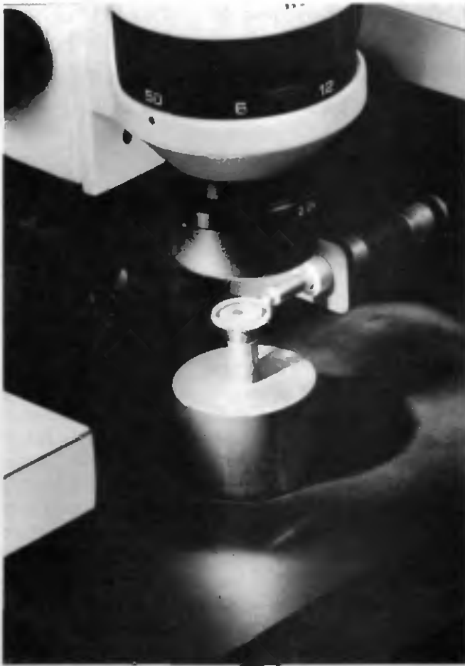
Fig. 6.2.3-4 UV curing of hybrid after centering
