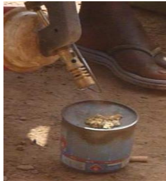
Picture 2-2 Burning the mercury-gold amalgam to recover the gold
