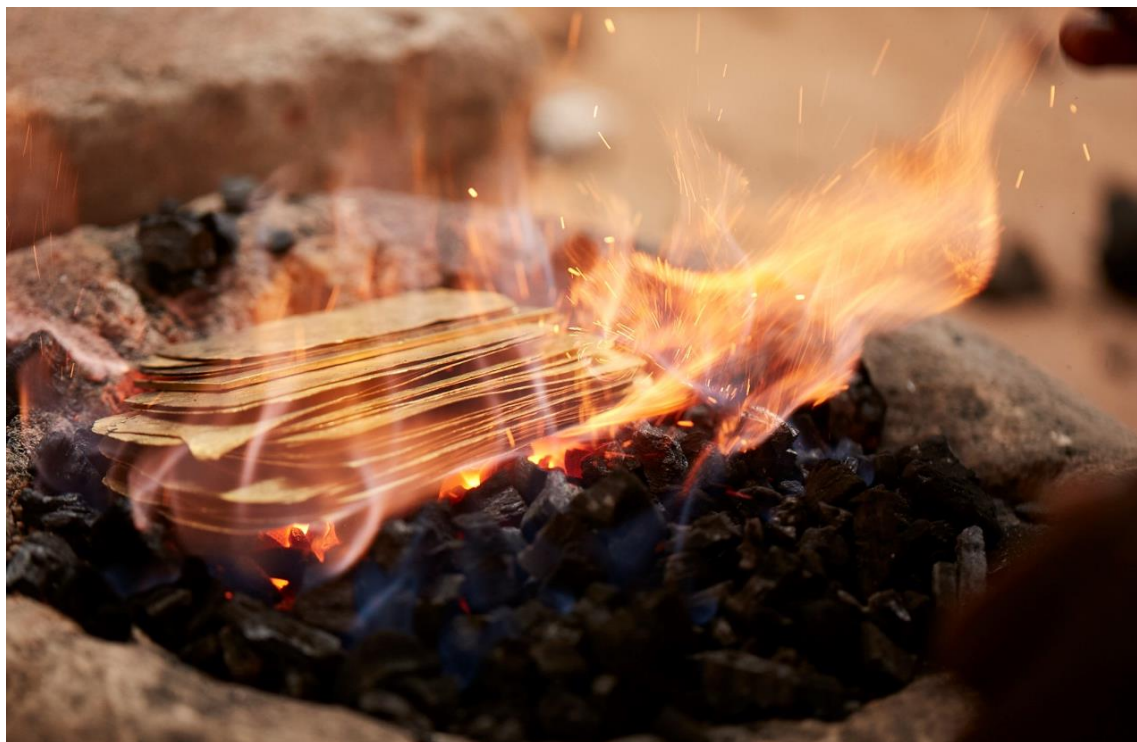
Picture 2-11 melting thin gold bars into a one-piece doré
