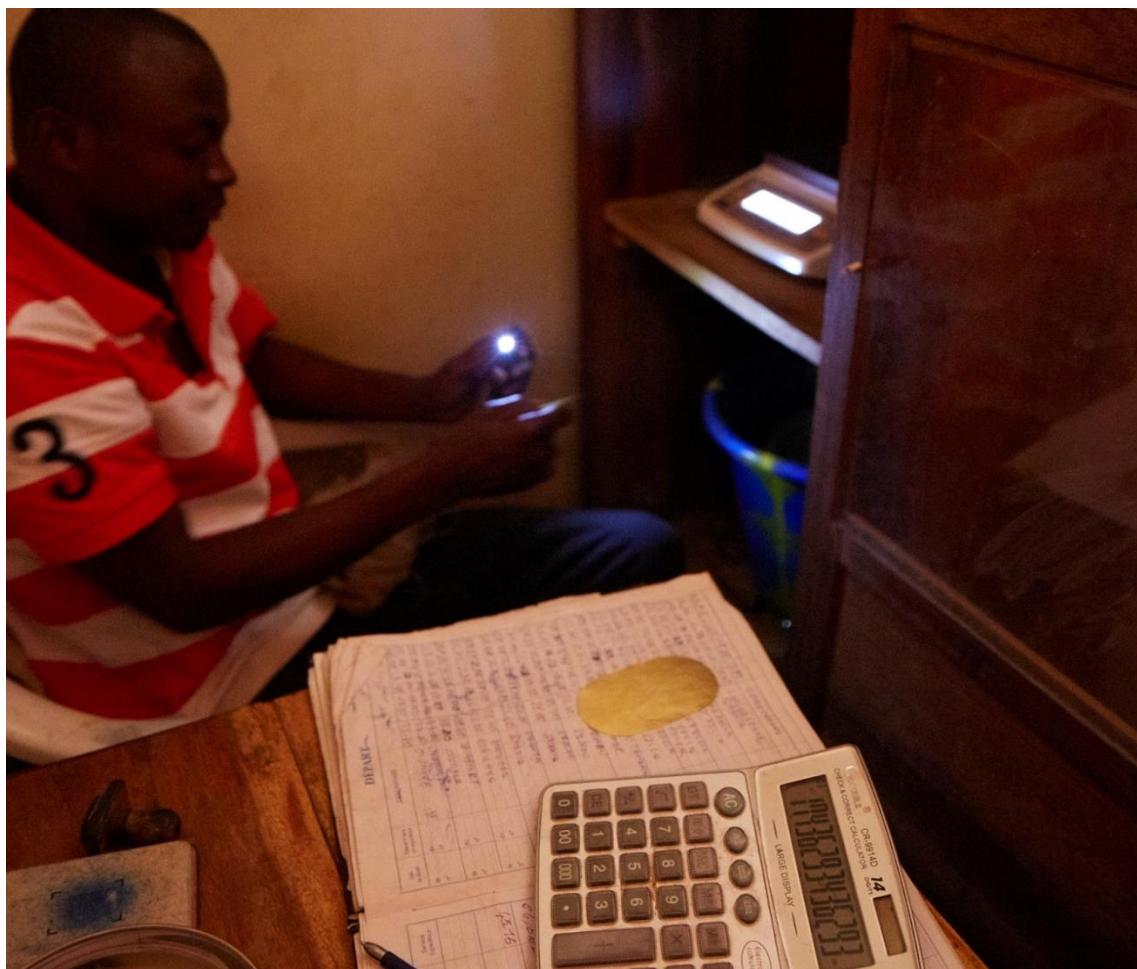
Picture 2-7 Densimetric weighing in a water bucket and titling of the thin gold bar (picture: Marion Bernet)
