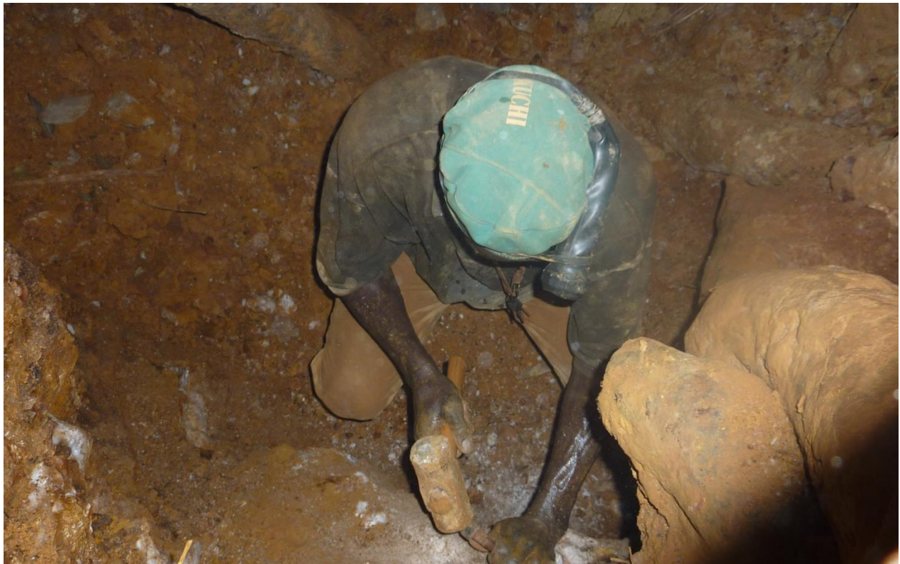
Picture 1-4 Kalayantigi cutting pieces of quartz rock in the horizontal tunnels at the deposit level (Mandiana, Guinea)
