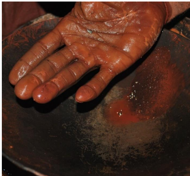
Picture 2-1 Mixing the heavy sands containing gold with mercury
