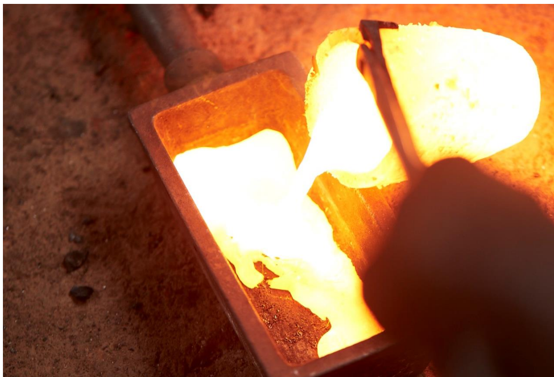
Picture 2-12 Making an approximately one kg doré
