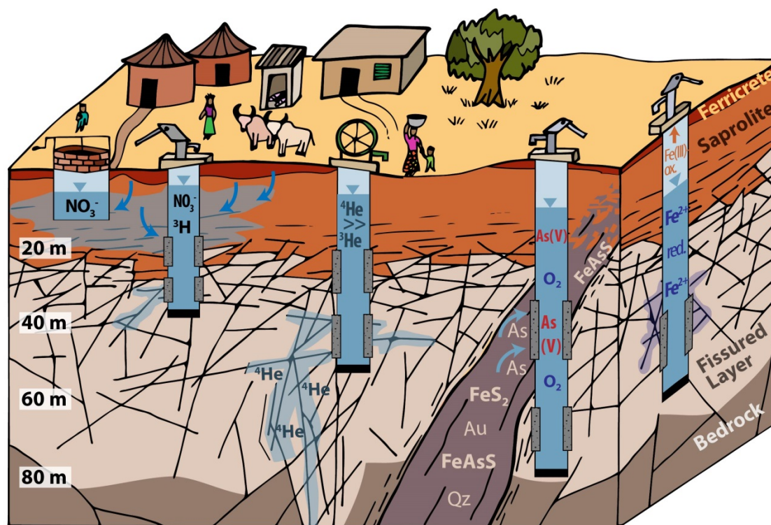
Fig. 3.13 Overview diagram illustrating the highly variable physical and chemical groundwater properties observed in the study area. From left to right: i) Groundwater in dug wells and shallow tube wells dominated by modern recharge and at times affected by pollution from settlements, livestock or agriculture. ii) Tube wells tapping groundwater with long residence times ( > 10^3 years, high ^4\text{He} concentrations) from fractures isolated from the modern water cycle, possibly with connections to deeper crustal zones. iii) Geogenic As contamination in wells directly dissecting mineralised zones, where As is released from sulphide minerals ( \text{FeAsS} , \text{FeS}_2 ) by oxidation and found in oxic groundwater as dissolved \text{As(V)} . iv) Locally mildly reducing conditions ( E_h < 300 mV) leading to high dissolved Fe concentrations. The diagram is not drawn to scale.
