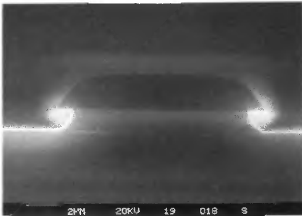
Fig. 2.13 Cross section of a polysilicon pattern which has been etched in a SF 6 /O 2 plasma (the photoresist is still on top).
