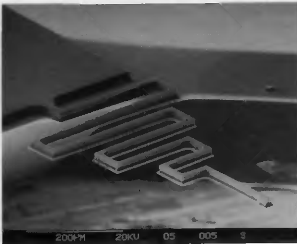
Fig. 2.22 Monocrystalline silicon cantilever with rectangular cross section and integrated tip fabricated by the process described in Fig. 2.21.
