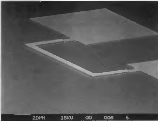
Fig. 2.4 SEM of an U-shaped free-standing P-doped polysilicon test structure for stress indication: large compressive stress would enlarge the bottom line of the "U" whereas tensile stress would diminish it. None of these effects has been observed.
