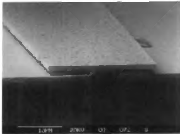
Fig. 2.7 Cross section (SEM) of a partly underetched phosphorus-doped polysilicon beam with CVD oxide as sacrificial layer.
